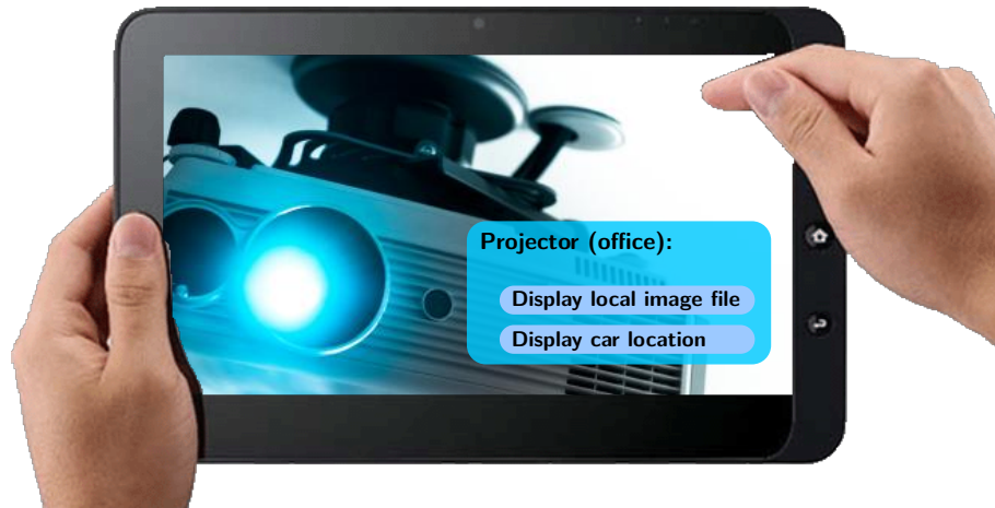
Figure 7.12: Using image recognition software and automatic deduction of user goals from RESTdesc descriptions (mock-up): a projector acts as a proxy for service mashups that it can form part of. In this case, the projector provides the service to either display an image that is stored on the tablet device, or to display the location of the user’s car on a map.
