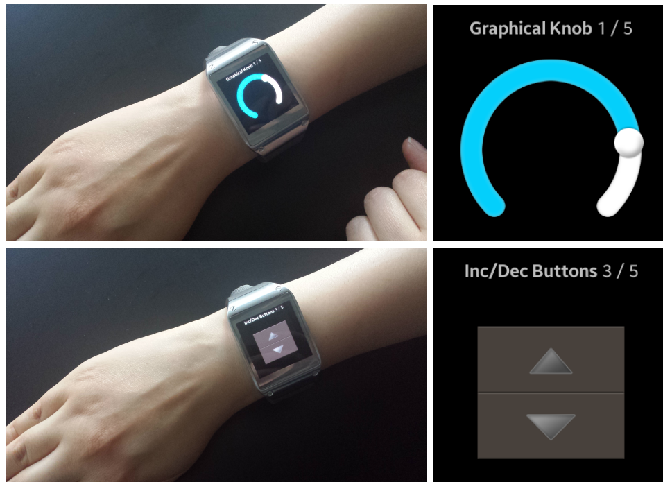
Figure 3.7: Interfaces for controlling the volume of a stereo set on a smartwatch (“set intensity”).
