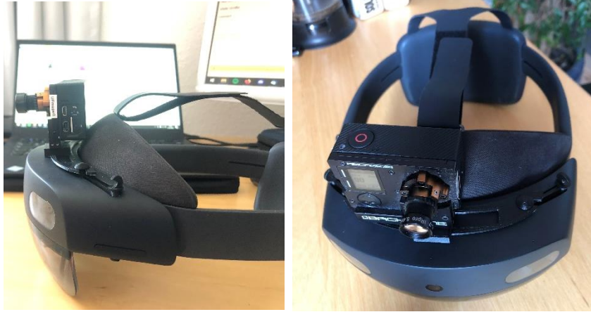
Figure 2: Mobile plant health visualizer consisting of an University of Florida Spectral Imager (modified GoPro Hero 4 Black) mounted onto a Microsoft HoloLens 2. [24]
