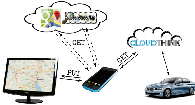
Fig. 7. By publishing semantic metadata that describes its interfaces, functionality of the CloudThink API (i.e., access to sensor values and actuators of connected vehicles) can be flexibly integrated with other local and remote Web services. In this example, a user instructs an interface device (in this case, a smartphone) to display the location of his car on a map that is shown on a nearby computer screen. A reasoner then finds the necessary HTTP requests to reach that goal and executes them.
