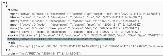
Figure 2: Exemplary data streams from the MQTT interface.
