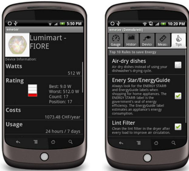
Figure 9. Android user interface: Device details (left), energy saving measures (right).
