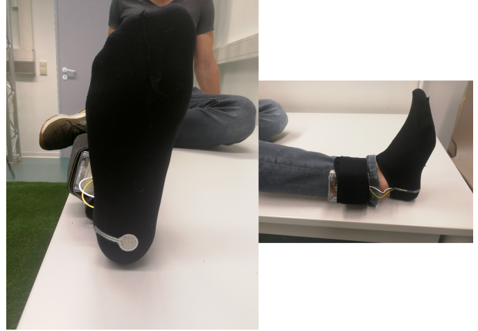
Figure 2: Attachment of the sensor at the heel and MCU at the ankle.
